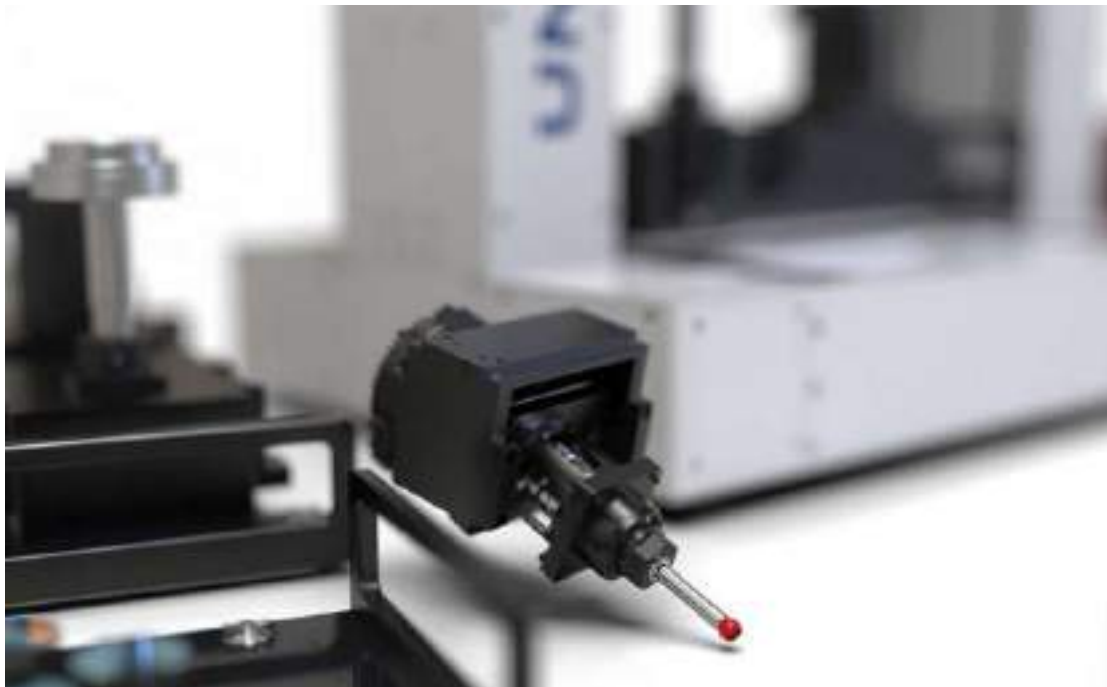
Traction module for use independently or together with the ROV module for servo controlled roll and slip configuration. Ideal for traction studies on bulk materials, coatings and on lubricants.
