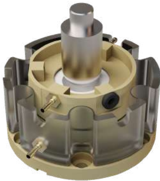
Test area with biofluid recirculation ports
