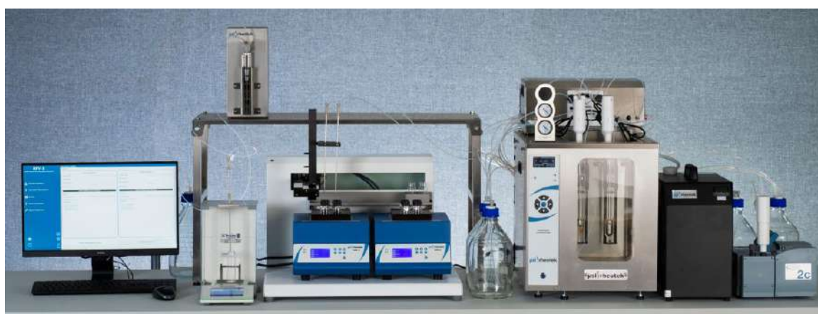
RPV-3 Auto Polymer Viscometer with two measurement positions and dual reaction blocks (with heating, stirring and cooling). See Appendix 20.7.
