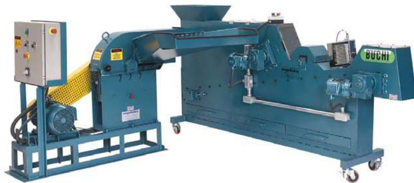
Fig.1.: BUCHI NIR-Online® Process Analyzer mounted on a conveyor machine for continuous measurements of Brix, POL, moisture and fiber in disintegrated sugarcane at the receival station.
