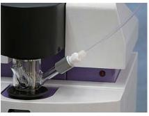
PTFE tubing connected to measuring cell for direct delivery from bottle-top dispenser for a safer aniline handling. PTFE tubing and fitting are not provided with aap-6. (option)
