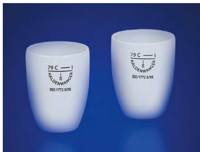
Haldenwanger crucibles shown before (left) and after (right) anneal testing. The result confirms the thermal stability of the glazing, even after multiple testing cycles.
