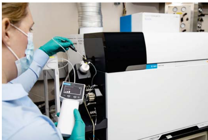
Figure 19. Checking for leaks at the nebulizer fittings on the Agilent 7900 ICP-MS.
