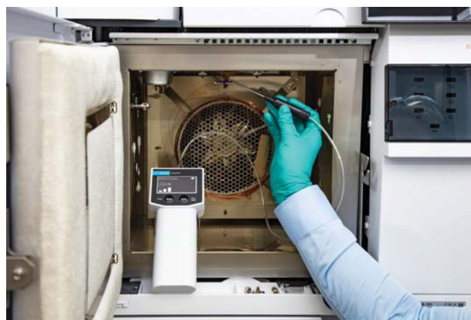
Figure 13. Checking for leaks at the GC inlet (A) and on Agilent Capillary Flow Technology (CFT) connections (B).
