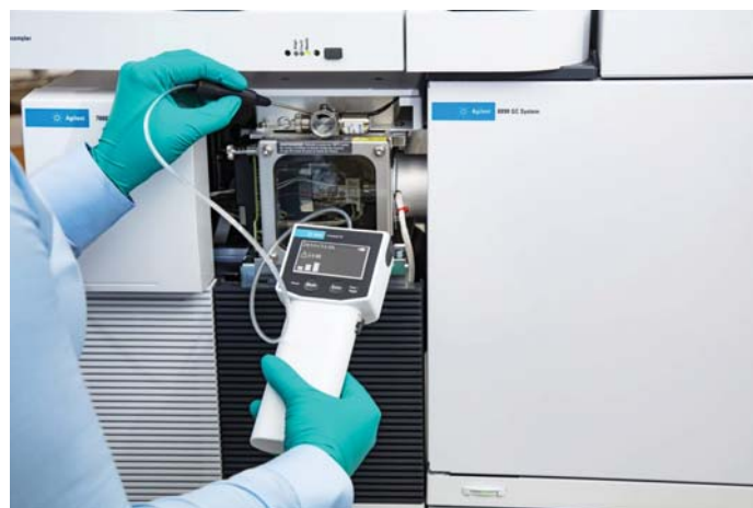
Figure 16. Checking for leaks on a GC/MS system at the mass spectrometer transfer line in the GC oven (A) and at the vent valve (B) on the mass spectrometer.
