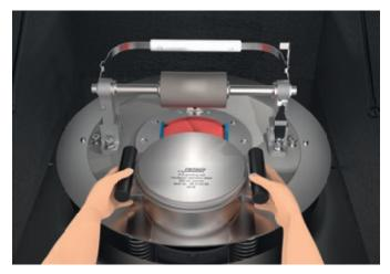
To mill, simply place the grinding set on the guide bar and push it into the end position.
