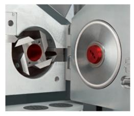
To ensure that P-15 continues to provide very stable running at high speeds, it comes fitted with double bearings on the shaft and in the cover. We have made the rotor blades reversible in order to double their service lives.
