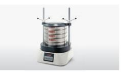
We recommend the A-18 Heavy Duty Analytical Sieve Shaker for particle size analysis and the fractionation of coarse-grained material.
