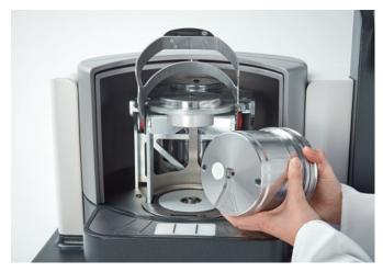
Insert the grinding bowl, lower the SelfLOCK handle and start the process: Grinding, mixing, homogenization and alloying in the FRITSCH P-5 premium line is that easy.
