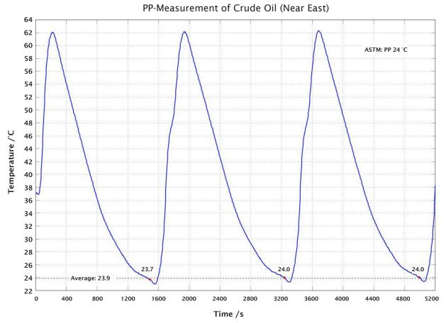
Measurement example for automatic repeated pour point measurement
