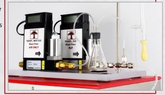
Tannas offers two TEOST® Mass Flow Controller models. The MHTurbo® Mass Flow Controller operates with the D7097 and D8447 tests, while the 33C Mass Flow Controller is utilized for all three TEOST tests (D6335, D7097, & D8447). Contact Tannas Co. for more details on these new Mass Flow Controller systems.
