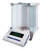
Analytical Electronic Balance with underplane support weight to position the support sample in the measurement area of the **MVS2pro**. The balance can be at 5 decimal places in grams. (d= 0,01 mg) The Balance is directly controlled by **MVS2pro** via USB.
