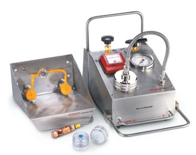
A bypass valve directs fuel through a filter cell containing the removable membrane filter or allows flushing of the sampler. Tested fuel may be routed to a flow line leading to a dump tank, without the need for buckets or containers.
