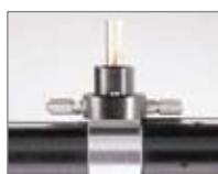
Sensor with air purge for dust measurements and filter test stands
